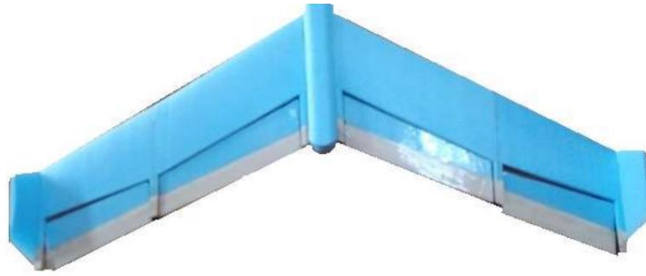
Figure 1121: Flying wing with only ailerons and elevators
